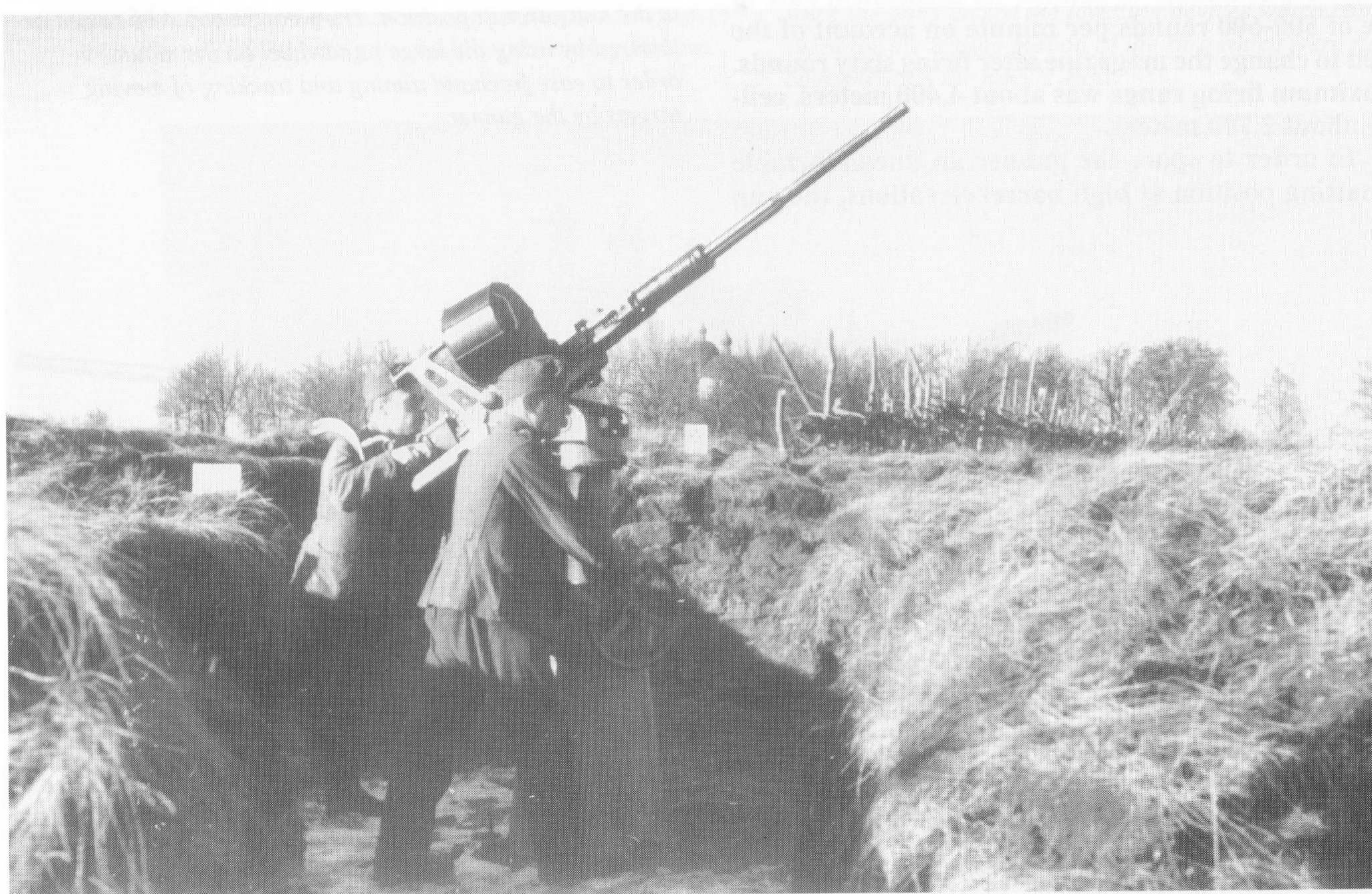
Both photos show the 20mm Oerlikon MK I on the MK II AA mount with adjustable-height gun mount in service with the navy. Above the gun is installed on a navy vessel, below in an emplacement ashore. The size of the large drum magazine is noteworthy.
