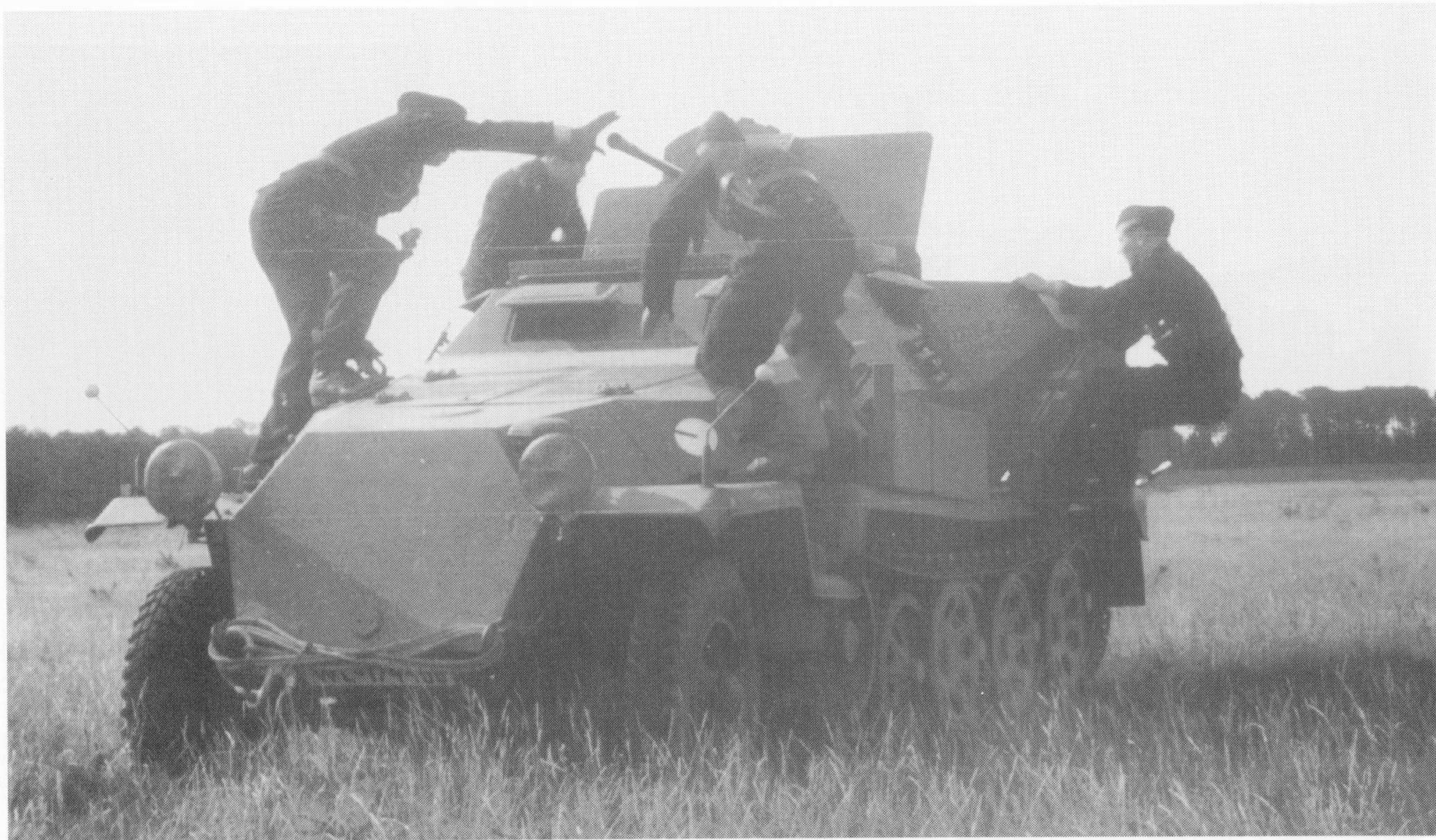
Here a 20mm Flak 38 is mounted on an armored troop carrier (Sd.Kfz. 251/17) of the "Hermann Göring" Division (note division emblem). The side panels could be folded down. The rifles were stowed in the box beside the driver's compartment.
