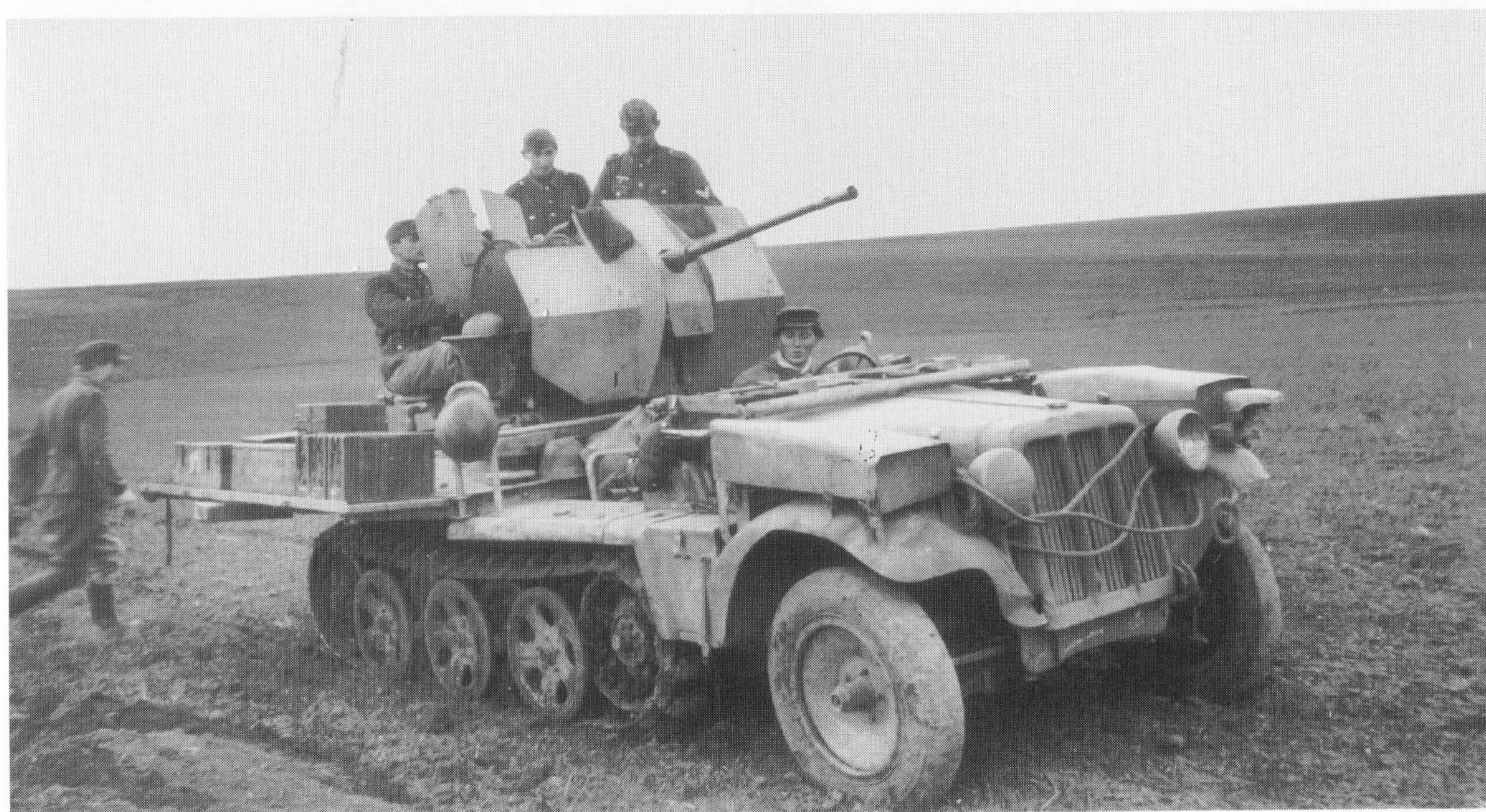
Here we see the Sd.Kfz. 10/4 light prime mover with a 20mm Flak 38. Boxes of ammunition are lined up on the sideboards, which have been folded down into the horizontal position. These served to enlarge the platform when the gun was in action. The boxes over the front fenders contain the gun crew's rifles (Karabiner 98k).
