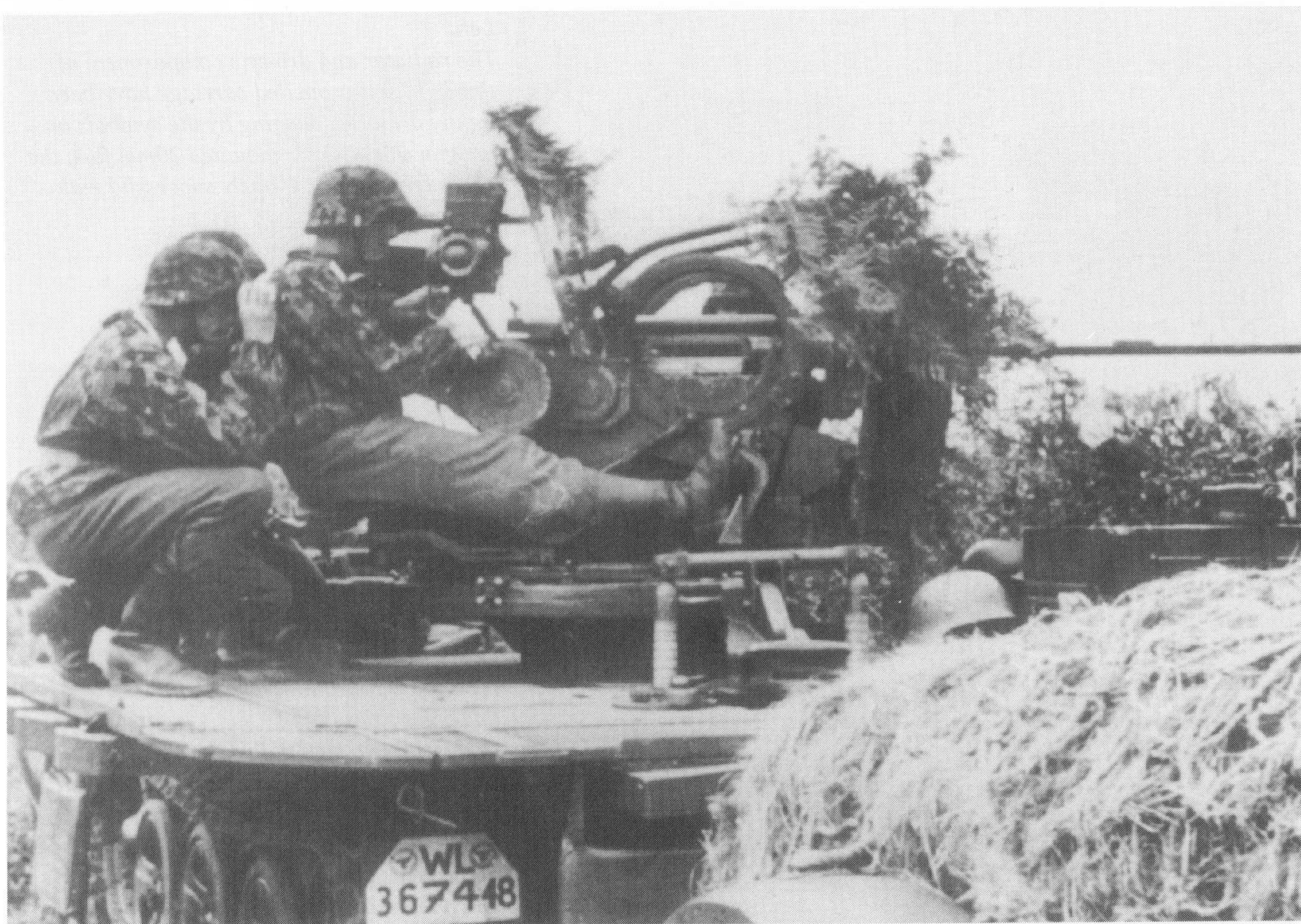
This 20mm Flak 38 is mounted on a camouflaged light prime mover, the Sd.Kfz. 10/4. The white collar tabs on the uniforms of the gun crew identify them as members of the "Hermann Göring" Division.
