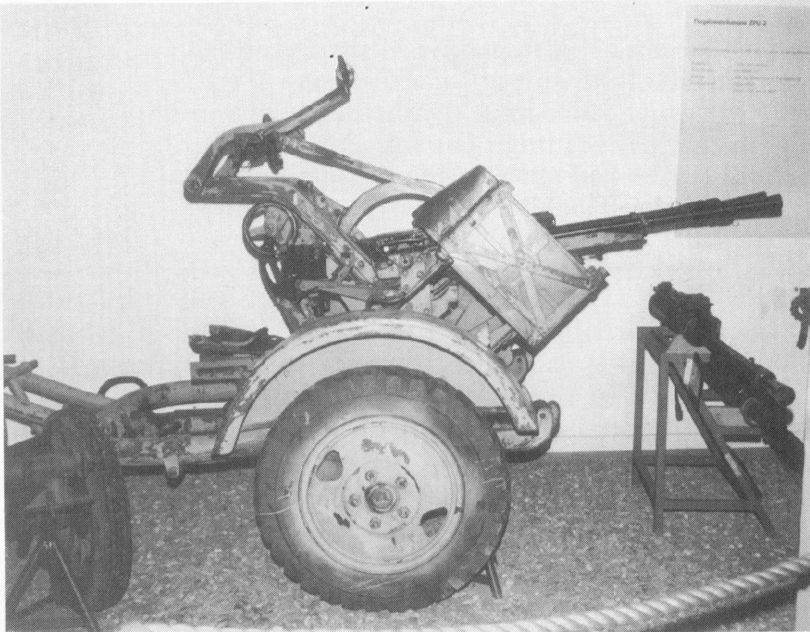
The three photographs on this page were taken in the Military Technology Study Collection in Koblenz. Above left is a 20mm Flak-Zwilling 38 in the M 44 double mount. Above right is a rare Flak-Zwilling 38 in a double mount, transportable on a single-axle Sonderanhänger 51 trailer.
