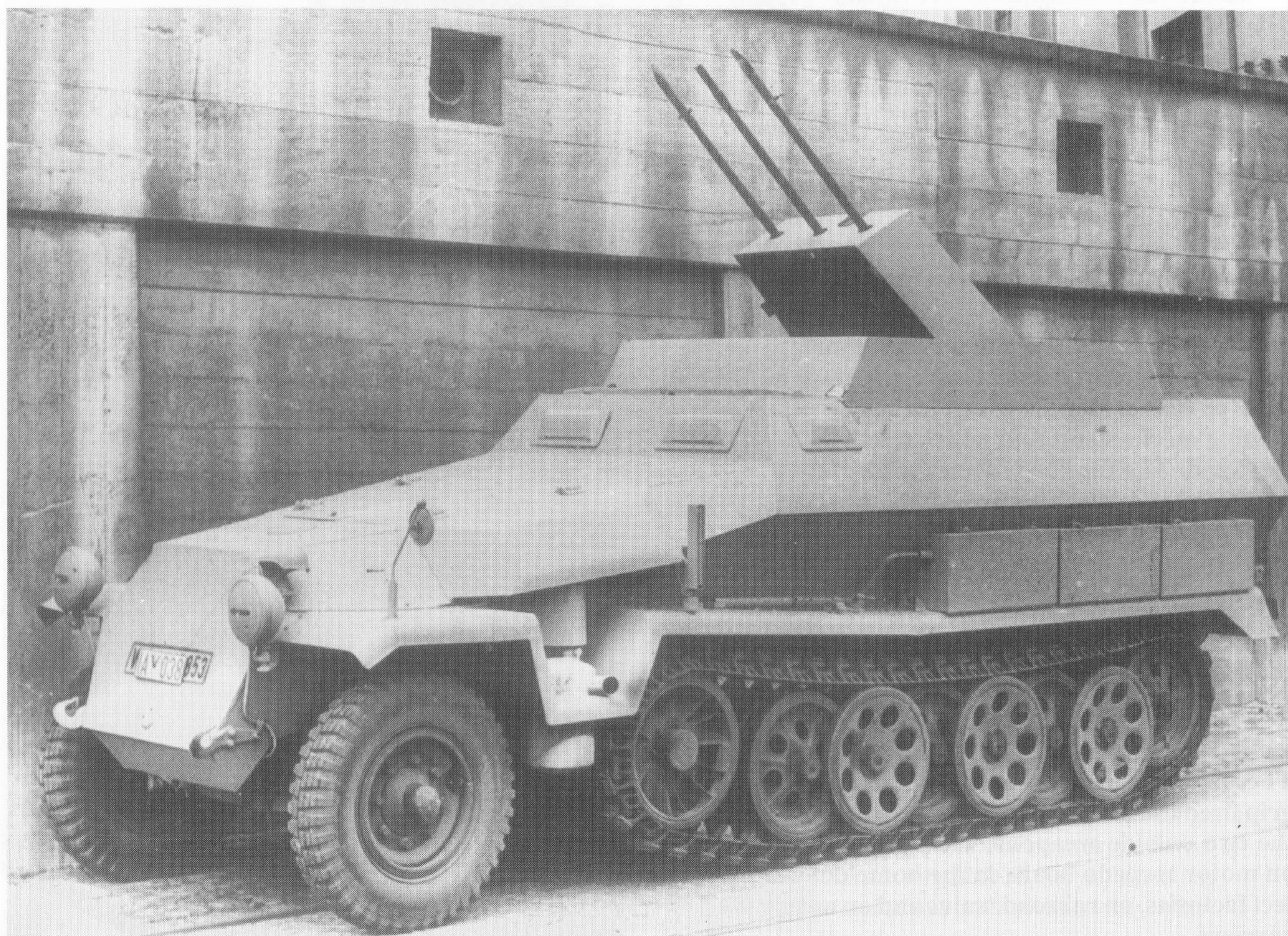
Below: An Sd.Kfz. 251/21 armored troop carrier with the anti-aircraft MG 151/ 20 cannon in a triple mount.
